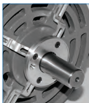
AEGIS® EP2400 Conductive Epoxy installation
