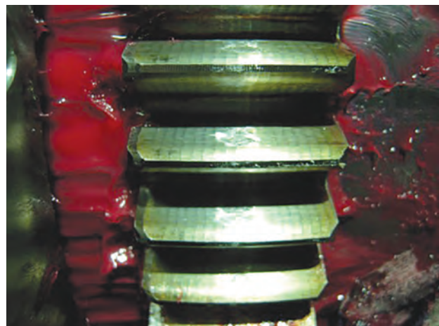
Tiger striping on the teeth of a gearbox caused by rotor ground current
